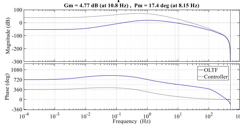
Figure 2: Controlled plant open loop response with controller
