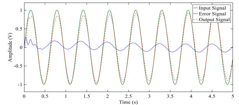
Figure 3: Time response of controlled plant with 2Hz demand signal
