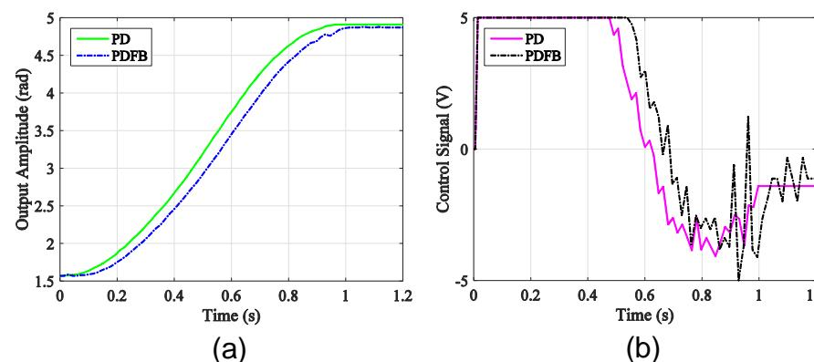
**Figure 2:** Experimental data obtained in the experiments done with the PD and the PDFB controllers applied to the rotary arm with the modified gains with a 3.14 rad angular displacement starting at 1.57 rad: (a) Output amplitude; (b) Control signal
