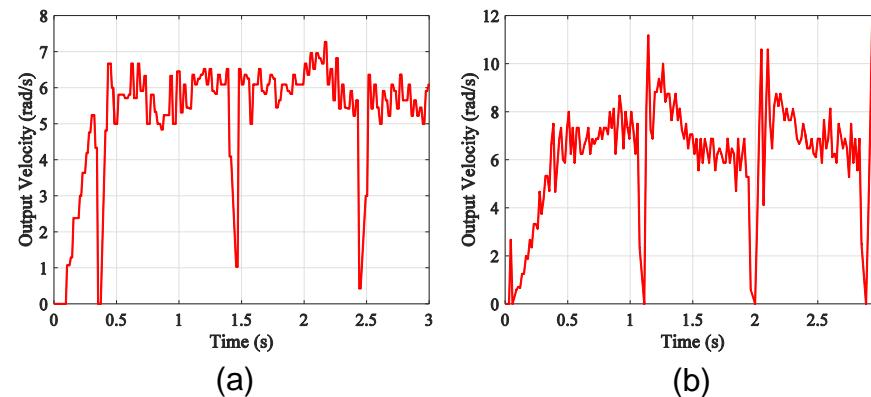
**Figure 1:** Output velocity obtained in the experiments done with the PI and the PID controllers applied to the rotary arm with a desired velocity of 6.28 rad/s: (a) PID controller; (b) PI controller
