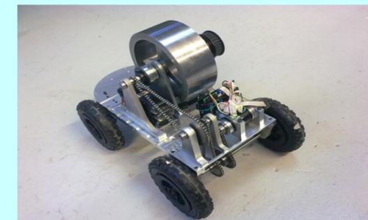
By following the driving procedures, an average settling time of 33.29 seconds has gained from the tests, while the theoretical value is 58 seconds. The error mainly came from the viscous friction of bearing rotations, which increased the vehicle deceleration by 1.7 times during flywheel driving process.
