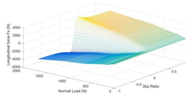
Figure 3: Longitudinal tyre forces as a function of slip ratio and normal load.
