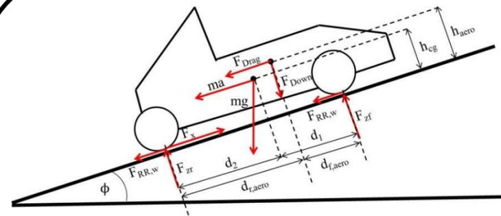
Figure 1: Forces on the FS car during straight-ahead driving.
