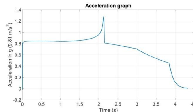
Figure 4: Example acceleration graph for a 75m acceleration.
