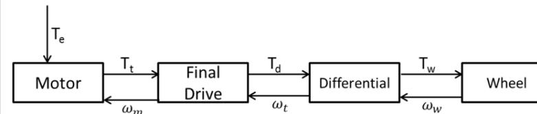
Figure 2: Power-train schematic depicting the flow of torque and velocity in the model.
