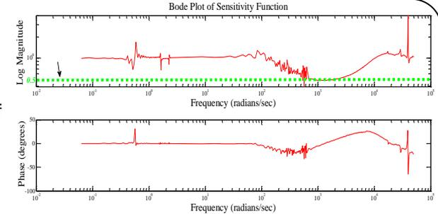
The best error rejection was within frequency region of  $100\text{rad/s}$ - $1000\text{rad/s}$  with an error rejection of  $-6\text{dB}$ . However, a resonance peak is still clearly seen from the bode plot above.
