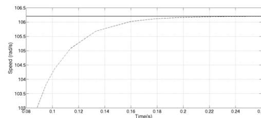
**Figure 3** – PI performance against non-linear plant
