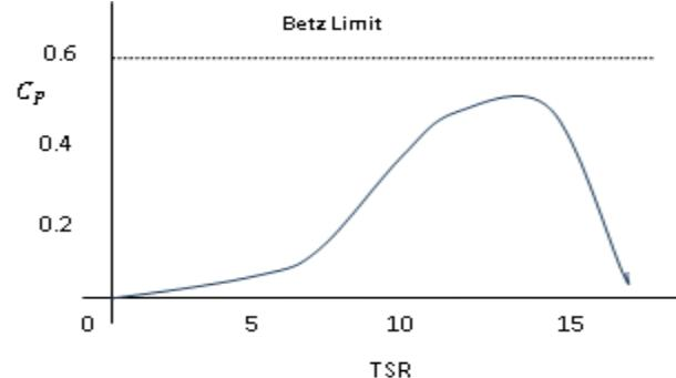
**Figure 2** – Typical relationship between TSR and coefficient of power
