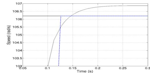
**Figure 4** – sliding mode (dashed line) vs PI control
