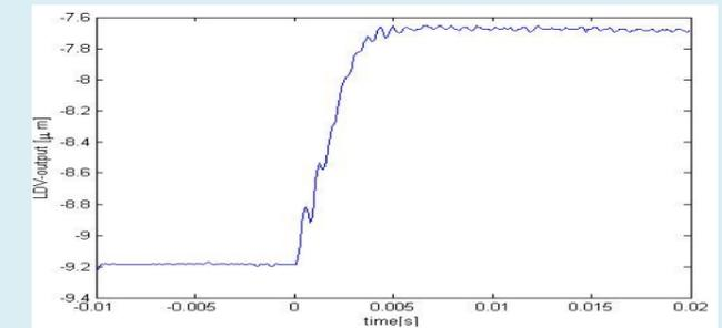
Fig above shows the output from LDV sensor, and natural frequency is found to be 1600 rads/s.
