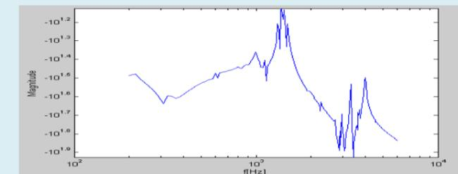
Figure above is the bode plot by PZT sensor output. A sharp peak in the magnitude plot indicates the resonance frequency which is at 1500rad/s.
