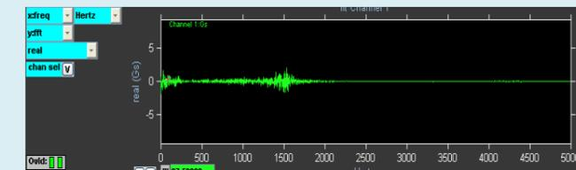
Figure above is a Fast Fourier transform of PZT output for PZT actuator subjected to random signal. A natural frequency about 1500 rads/s is found.
