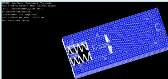
The figure shows a finite element analysis of one of the design of the stage when the platform is under 100N of actuator force.
