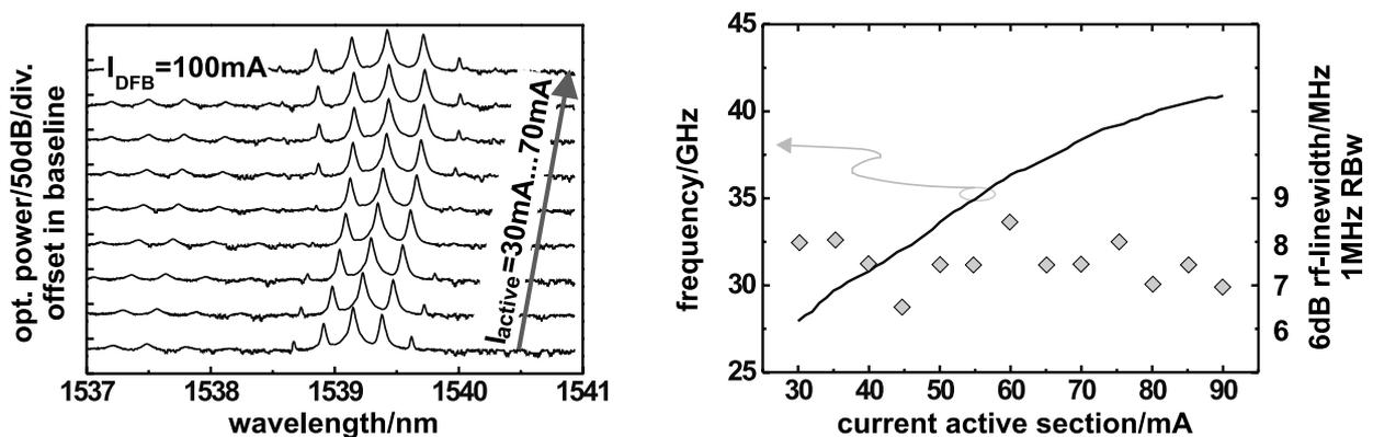
Fig. 2. Optical spectra for different microwave frequencies (left). Right side: Continuous frequency tuning range by increasing the current in the active section. Diamonds show the linewidth of rf-spectra.
