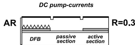
Fig. 1. Scheme of the DFB with an amplifying mirror.
