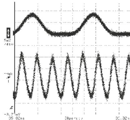
Fig. 3. Microwave source locked to a 10Gbit/s subharmonic PRBS  $2^7-1$  pulse train.
